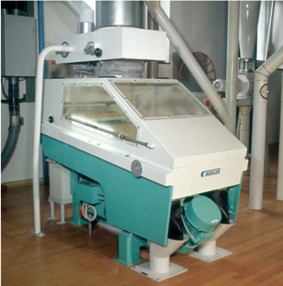
Destoner MTSC. Execution with one screen deck.
